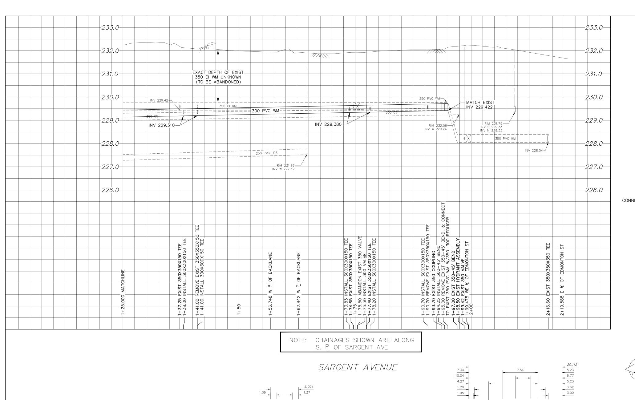
\_ 300 PVC WM INSTALL 300X300X150 TEE -INSTALL 150 VALVE 150 PVC SERVICE -CONNECT TO EXIST 150 AC SERVICE W/COUPLING -EXIST 150 AC SERVICE — S ₧ OF SARGENT AVE
