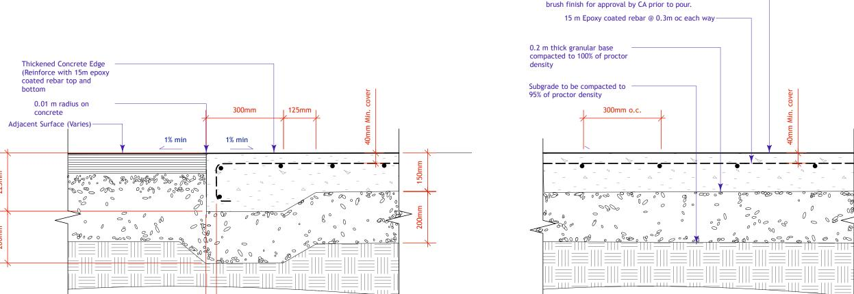
**Concrete Notes** 1. Contractor to provide shop drawings showing foundation and grounding details for pool toys stamped by a professional engineer registered to practice in Manitoba. 2. Concrete to be 32 mpa at 28 days Maxiumum agg. size 19 mm 4. Air Entraining 6-9% 5. All reinforcing steel to be epoxy coated 6. Exposure Class F1 7. Contractor to provide density testing of the sub-base and the granular base course. Results of testing to be sent directly from the testing lab to the Contract
