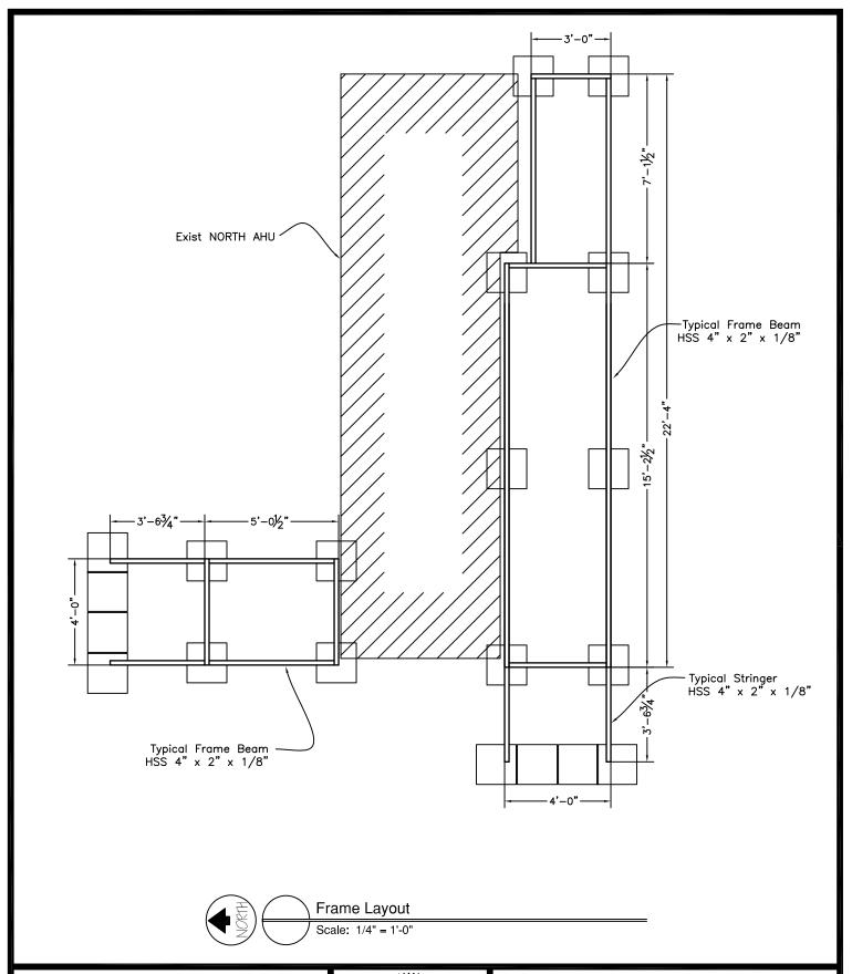
SK-8 (R-1) New Roof Top AHU Platform Pan Am Pool 25 Poseidon Bay Winnipeg, Manitoba
