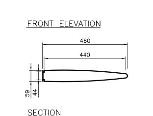
SIDE ELEVATION SIGN BOX TO HAVE INTEGRAL STAINLESS STEEL TOP AND BOTTOM. PROVIDE DRAIN HOLES VINYL MATERIALS / GRAPHIC PRODUCTION TO BE CONSISTENT WITH LOCALLY AVAILABLE (MANITOBA)
