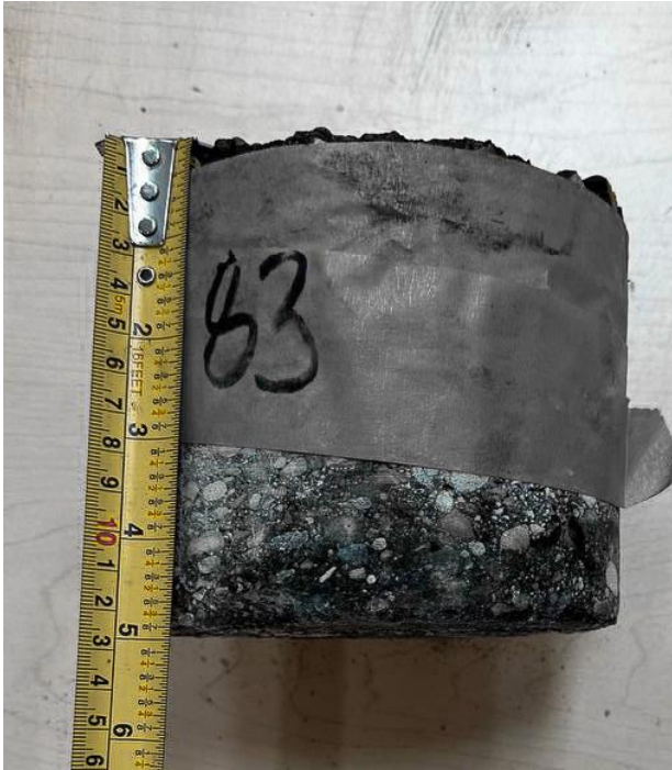
Montclair Bay, WBL ++ , Core 83 (Asphalt Thk 120mm)
