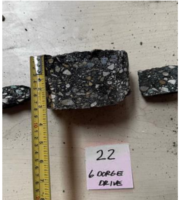
Dorge Drive, NBL ++ , Core 22 (Asphalt Thk 75mm)
