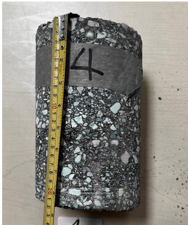
Brady Road, SBL + , Core 4 (Asphalt Thk 217mm)
