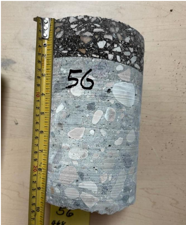
Scurfield Blvd, NBL ++ , Core 56 (Asphalt Thk 50mm, Concrete Thk 190mm)
