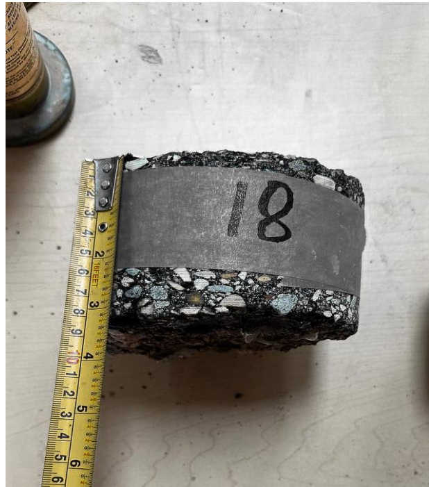
Dorge Drive, EBL ++ , Core 18 (Asphalt Thk 72mm)
