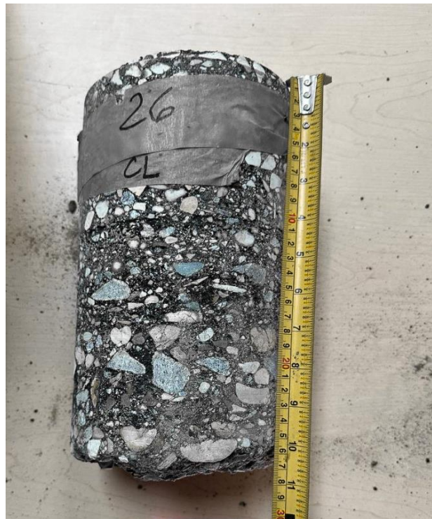
Turnbull Drive, SBL + , Core 26 (Asphalt Thk 265mm)
