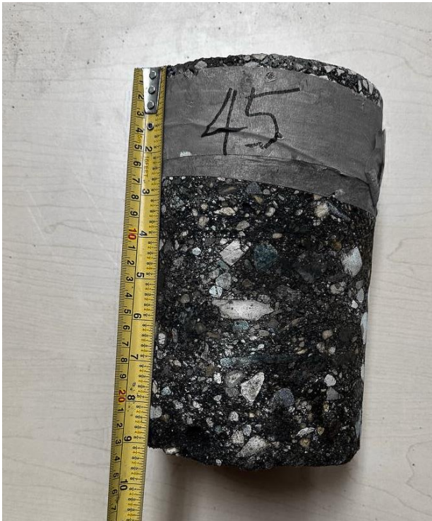
Turnbull Drive, NBL + , Core 45 (Asphalt Thk 325mm)
