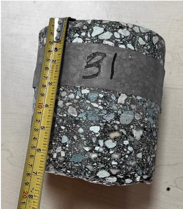
Turnbull Drive, NBL + , Core 31 (Asphalt Thk 170mm)
