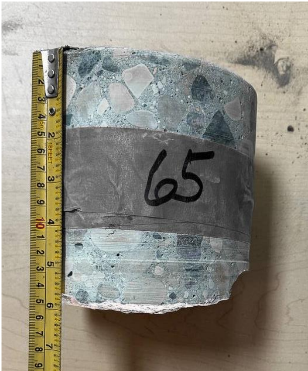
Sandstone PI, Outer Lane ++ , Core 65 (Concrete Thk 140mm)
