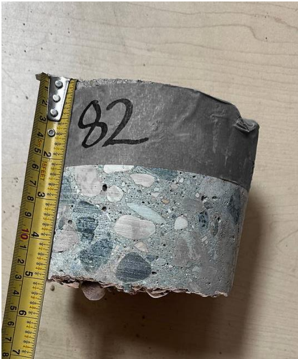
Greensboro Sq, Outer Lane ++ , Core 82 (Concrete Thk 120mm)
