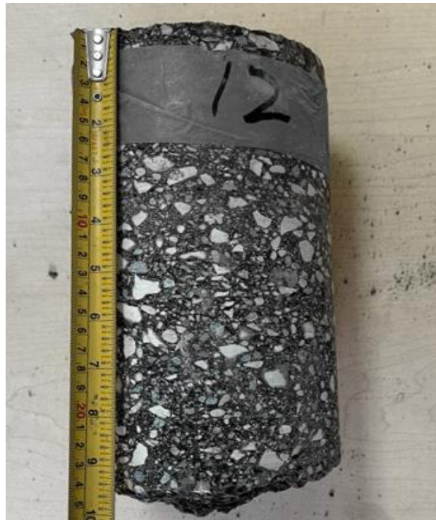
Brady Road, SBL + , Core 12 (Asphalt Thk 240mm)
