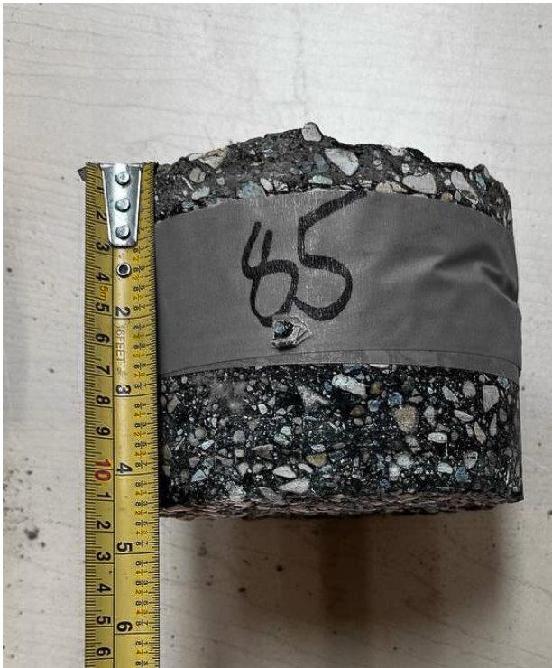
Montclair Bay, EBL ++ , Core 85 (Asphalt Thk 110mm)
