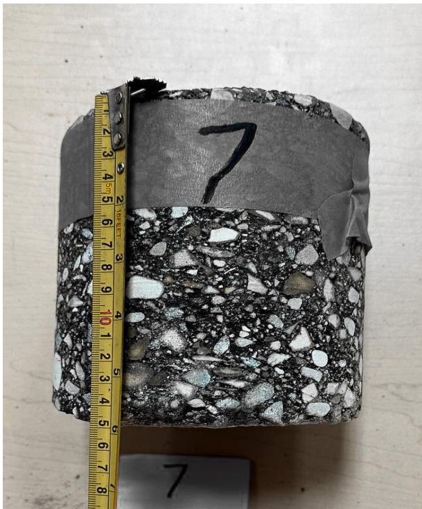
Brady Road, NBL + , Core 7 (Asphalt Thk 145mm)
