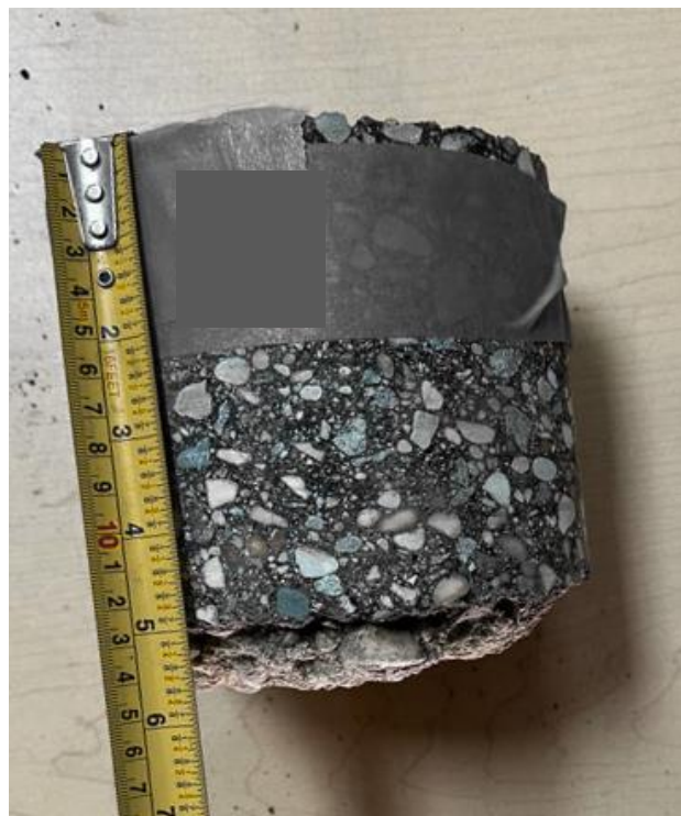
Greensboro Bay, WBL ++ , Core 79 (Asphalt Thk 125mm)
