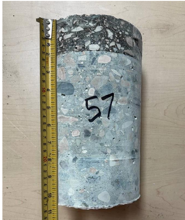
Scurfield Blvd, NBL ++ , Core 57 (Asphalt Thk 50mm, Concrete Thk 220mm)
