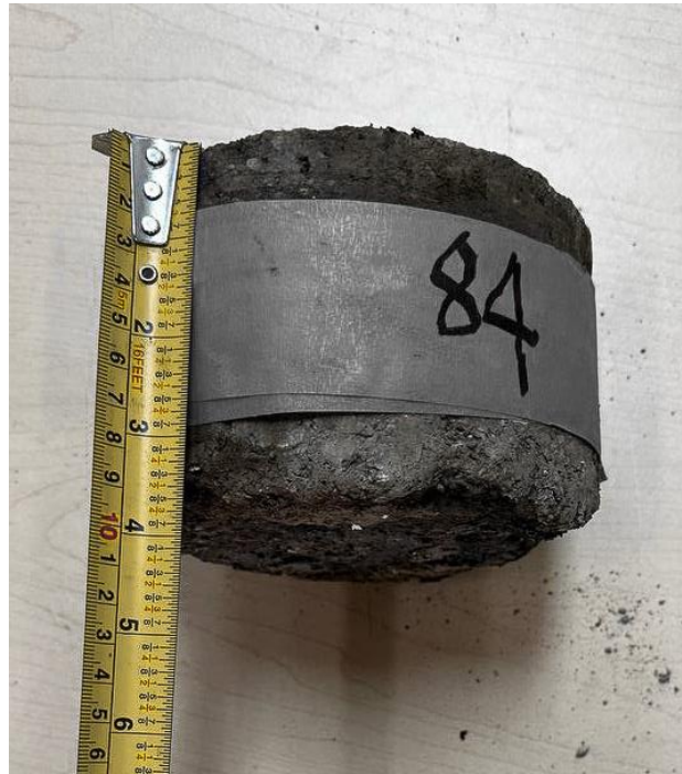
Montclair Bay, WBL ++ , Core 84 (Asphalt Thk 80mm)
