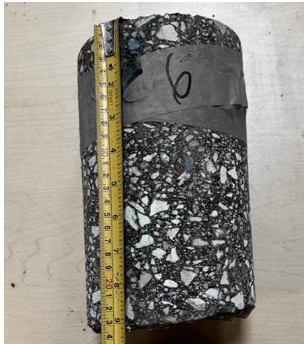
Brady Road, SBL + , Core 6 (Asphalt Thk 235mm)
