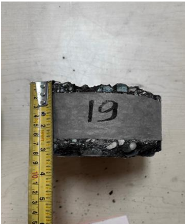
Dorge Drive, WBL ++ , Core 19 (Asphalt Thk 70mm)
