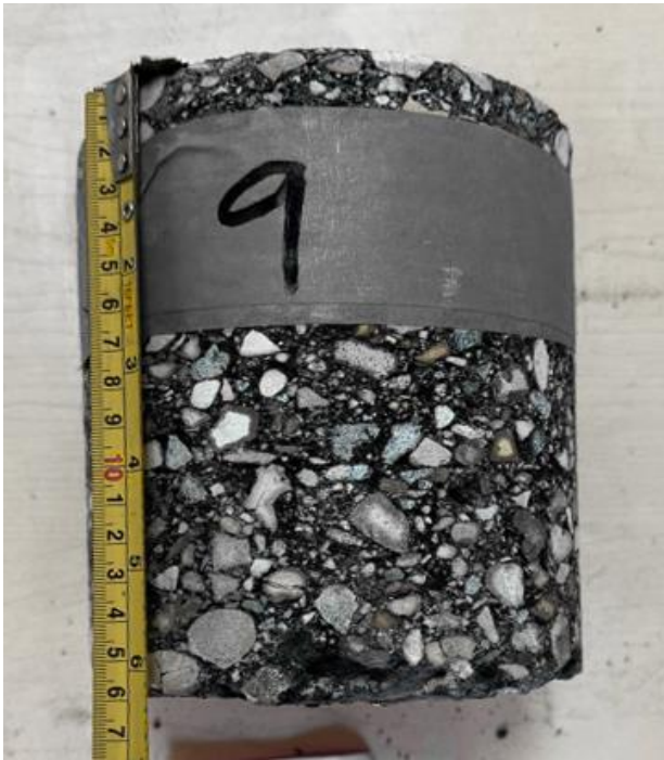
Brady Road, NBL + , Core 9 (Asphalt Thk 157mm)
