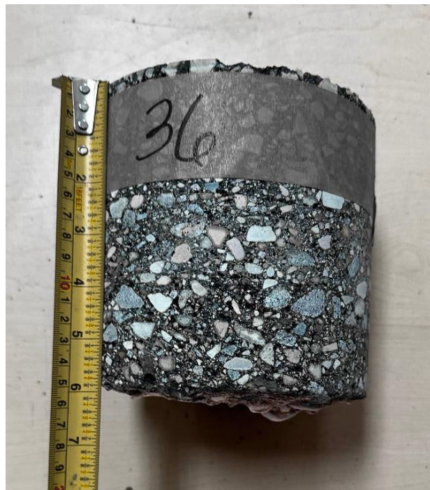
Turnbull Drive, NBL + , Core 36 (Asphalt Thk 150mm)
