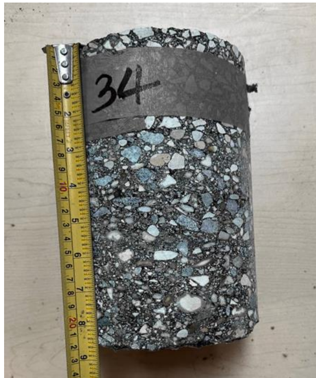
Turnbull Drive, NBL +++ , Core 34 (Asphalt Thk 220mm)
