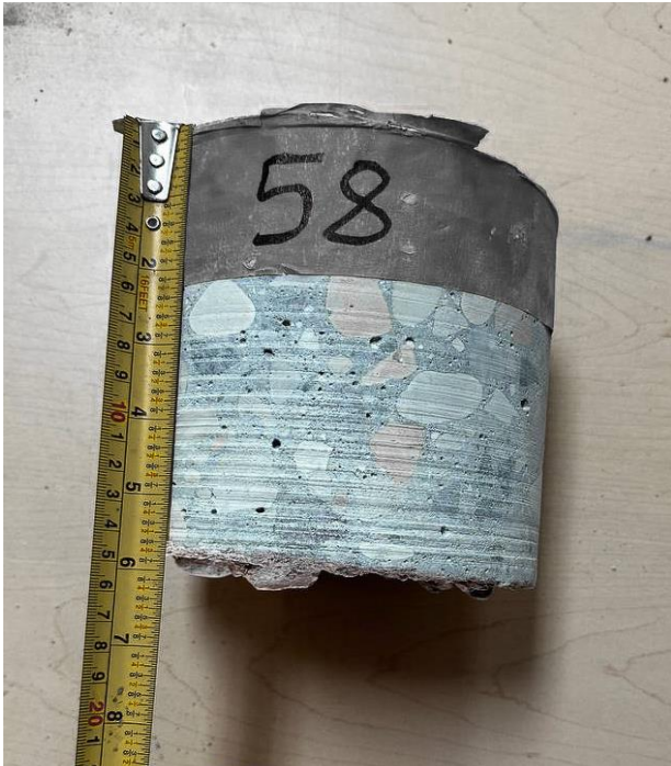
Scurfield Blvd, Inner Lane ++ , Core 58 (Concrete Thk 140mm)
