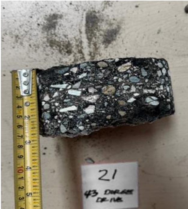
Dorge Drive, WBL ++ , Core 21 (Asphalt Thk 70mm)
