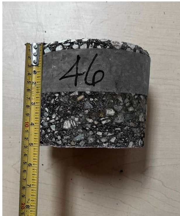
Turnbull Drive, NBL +++ , Core 46 (Asphalt Thk 125mm)
