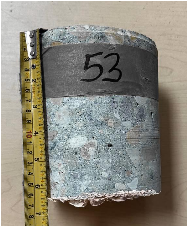
Fleetwood Rd, WBL ++ , Core 53 (Concrete Thk 160mm)
