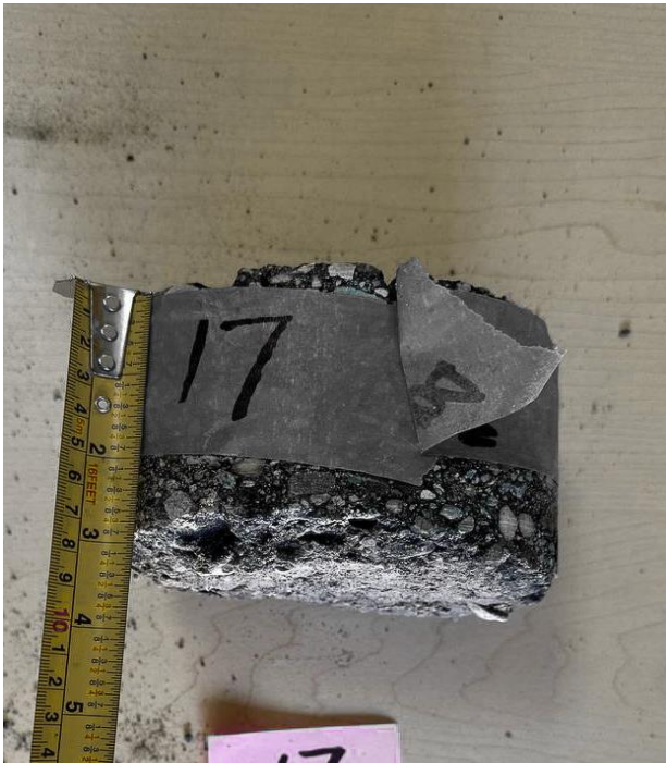
Dorge Drive, NBL ++ , Core 17 (Asphalt Thk 72mm)
