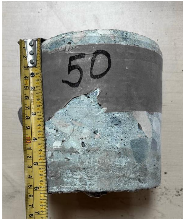
Westbourne Cr, SBL ++ , Core 50 (Concrete Thk 155mm)
