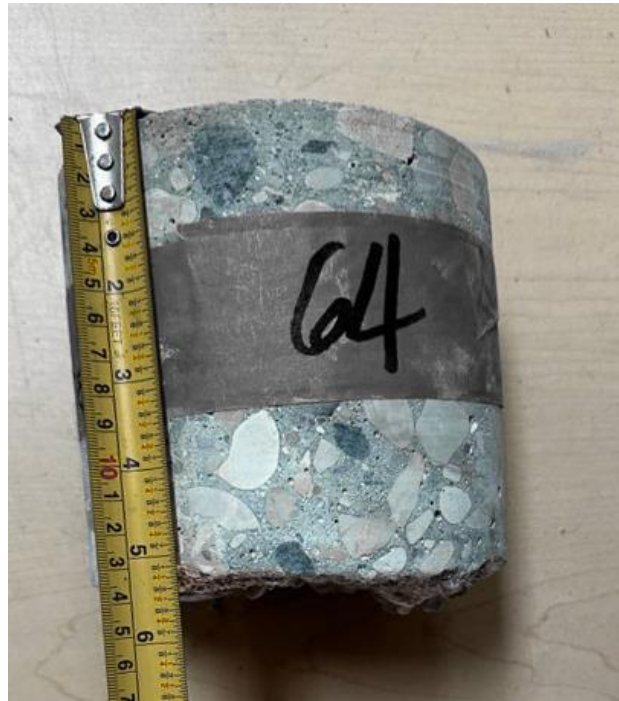
Sandstone PI, Inner Lane ++ , Core 64 (Concrete Thk 135mm)
