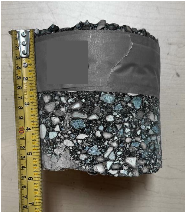
Greensboro Bay, NBL ++ , Core 76 (Asphalt Thk 140mm)
