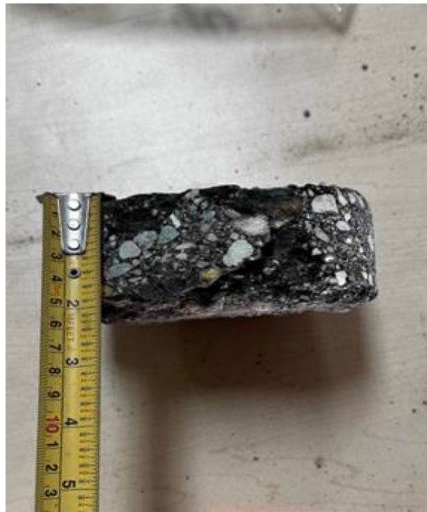
Dorge Drive, EBL ++ , Core 20 (Asphalt Thk 50mm)
