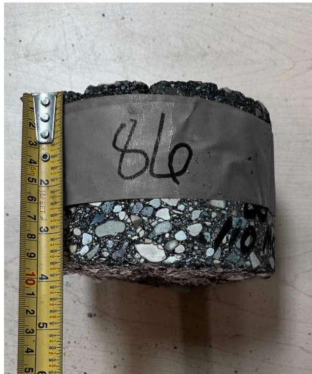
Montclair Bay, SBL ++ , Core 86 (Asphalt Thk 90mm)
