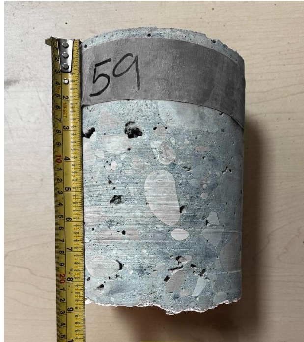
Scurfield Blvd, NBL ++ , Core 59 (Concrete Thk 220mm)
