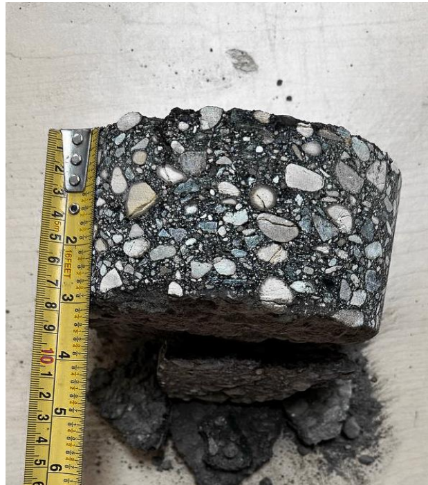
Augusta Dr, SBL ++ , Core 67 (Asphalt Thk 100mm)
