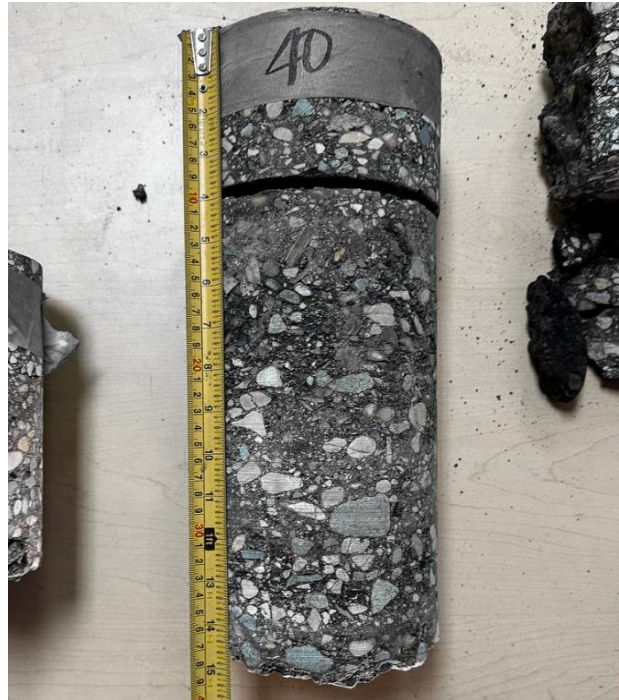
Turnbull Drive, SBL + , Core 40 (Asphalt Thk 365mm)
