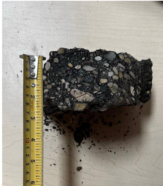
Providence PI, NBL ++ , Core 74 (Asphalt Thk 50mm)
