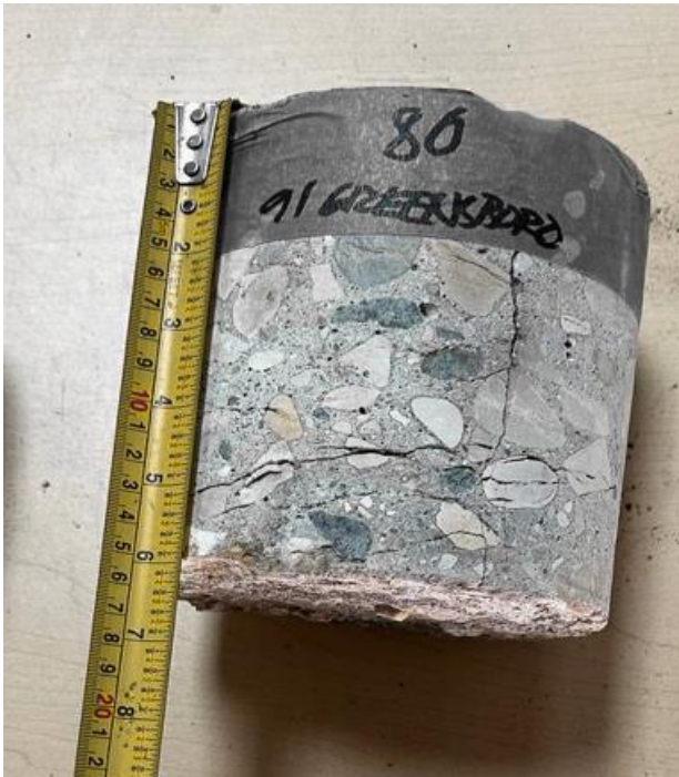
Greensboro Bay, NBL ++ , Core 80 (Concrete Thk 155mm)
