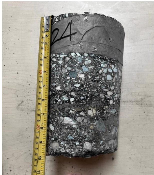
Turnbull Drive, NBL + , Core 24 (Asphalt Thk 170mm)
