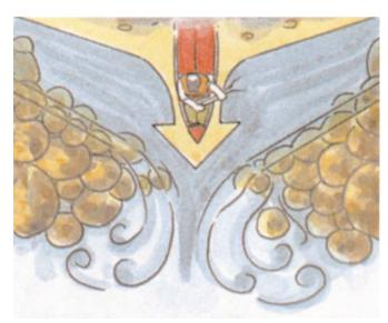
Figure 6: Although water is squeezed through the stone riffles, they allows fish to pass up or down stream.
